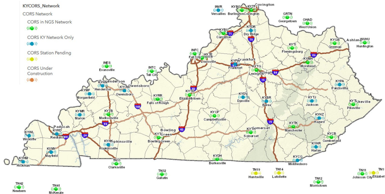
Figure 1.5.1 Kentucky CORS (KyCORS) network with stations in surrounding states. Green symbols represent stations within the NOAA CORS Network (NCN) and blue symbols represent stations within the KyCORS network only. (KYTC, 2019)
