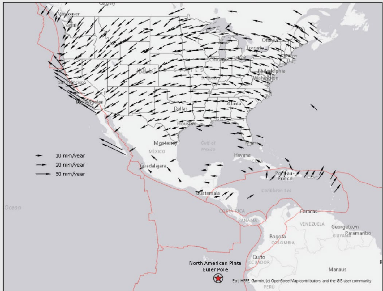
Figure 1.6.1 Vectors of horizontal velocity at select Continuously Operating Reference Stations (CORSs) on multiple tectonic plates determined by NGS, as well as an associated Euler pole solution for the North American Plate. (NGS 2021)
